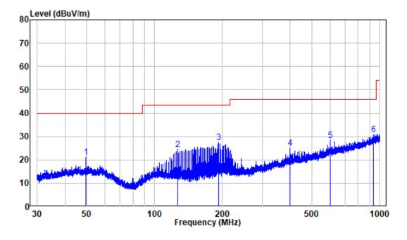
Site : chamber Condition: 3m VERTICAL Job No. : SZNS220303-07023E-RF Test Mode: Working
