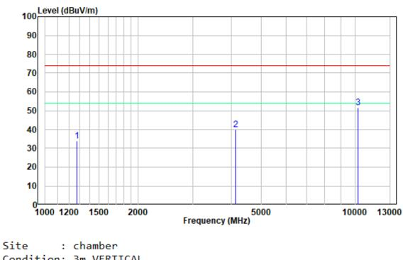
Site : chamber Condition: 3m VERTICAL Job No. : SZNS220303-07023E-RF Test Mode: Working
