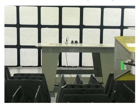
Radiated Emissions – Rear View (Above 1 GHz)
