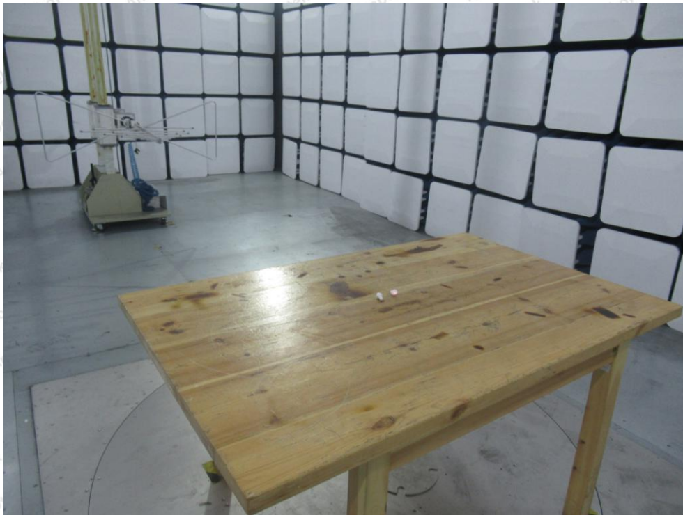
Photo of Radiation Emission Test
