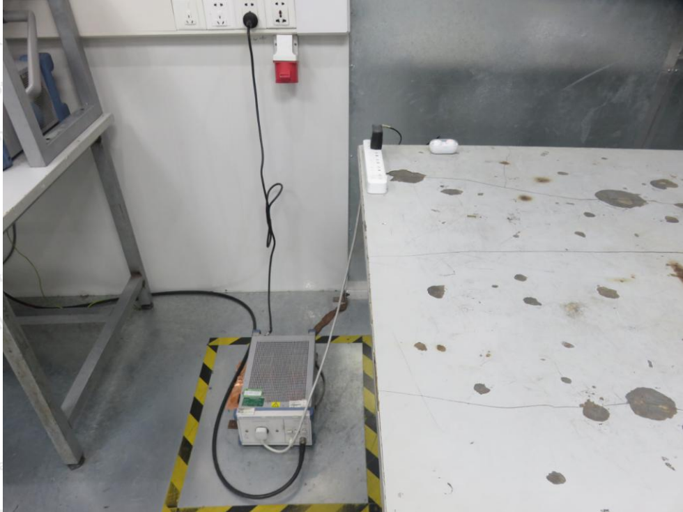
Photo of Conducted Emission Measurement
