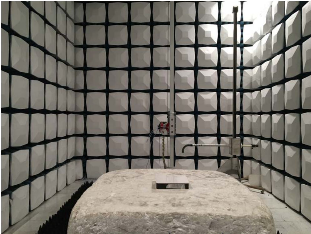
Description: Radiated Emission Test Setup for 1~18GHz
