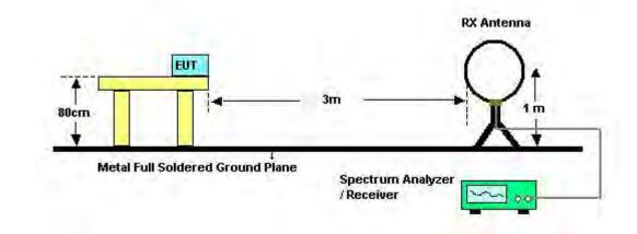
For Radiated Emissions: 30MHz~1GHz
