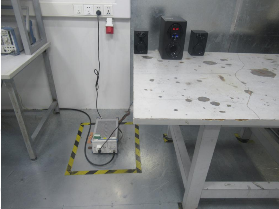
Photo of Conducted Emission Measurement
