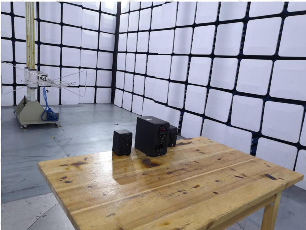
Photo of Radiation Emission Test
