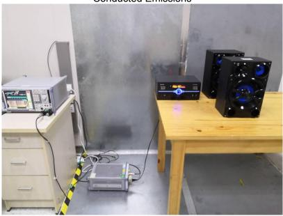
Radiated Spurious Emissions Test Frequency From Below 30MHz
