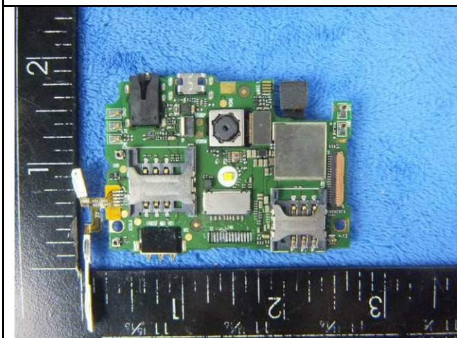
Mainboard with Shielding - Front View
