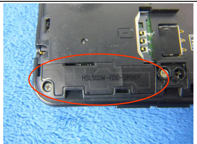
LTE - Antenna View
