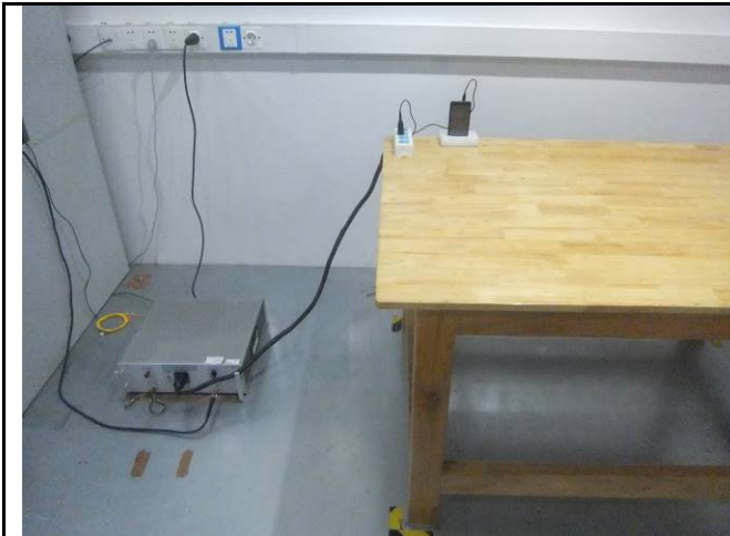
Conducted Emissions Test Setup Front View
