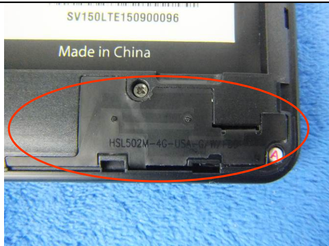
GSM/PCS/UMTS-FDD Antenna View
