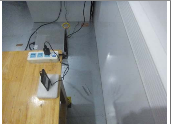
Conducted Emissions Test Setup Side View
