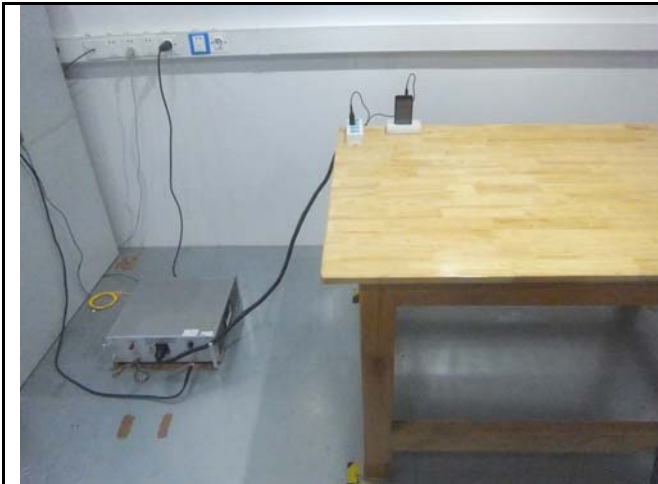
Conducted Emissions Test Setup Front View
