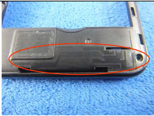
GSM/PCS/UMTS-FDD Antenna View
