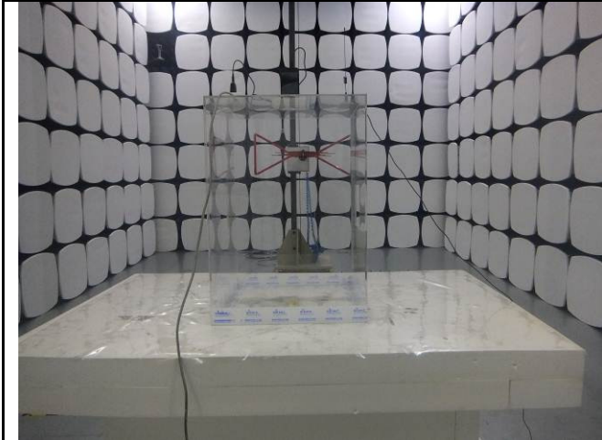
Radiated Spurious Emissions Test Setup Below 1GHz
