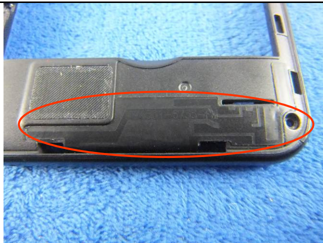
GSM/PCS/UMTS-FDD Antenna View
