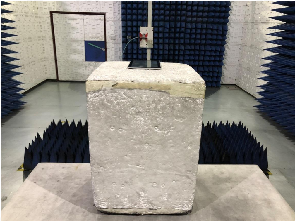
FCC RADIATED EMISSION TEST SETUP ABOVE 1GHZ
