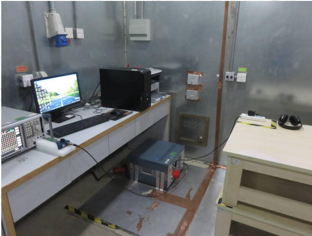
FCC RADIATED EMISSION TEST SETUP
