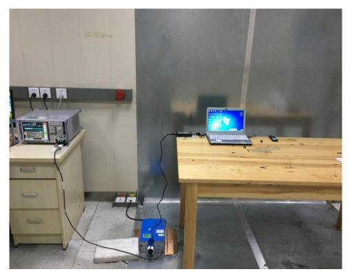
FCC RADIATED EMISSION TEST SETUP
