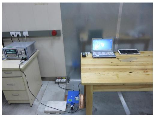
FCC RADIATED EMISSION TEST SETUP
