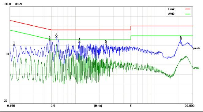
Site: Conduction Phase: N Temperature: 22.5 Limit: FCC Class B Conduction(QP) Power: Humidity: 50.6 %
