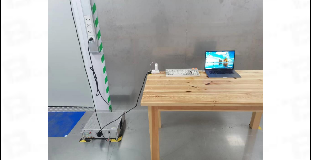
Conducted Emission at AC power line
