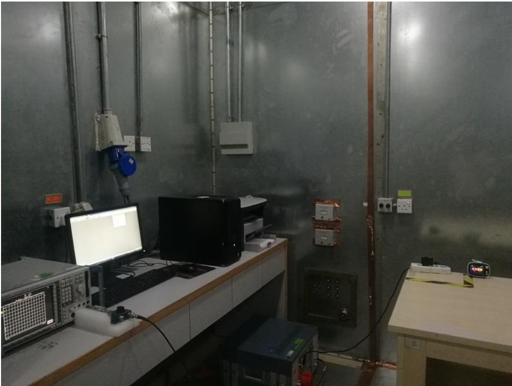
FCC RADIATED EMISSION TEST SETUP
