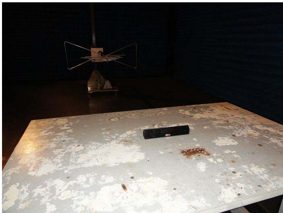
Radiated Emission Test Setup:
