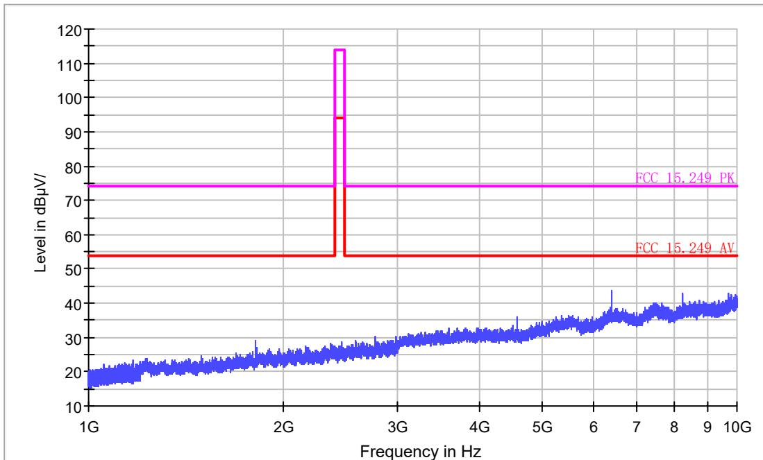
Transmitting at 916MHz, above 1GHz, Horizontal
