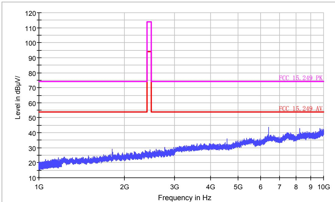
Transmitting at 916MHz, above 1GHz, Horizontal
