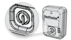
To turn on the Player Tag, press the power button in the middle of the device.
