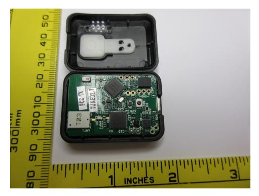
**1.2** EUT – Open Case View Main Board Top view
