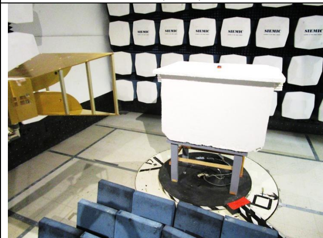
Radiated Emissions (>1GHz) – Front View
