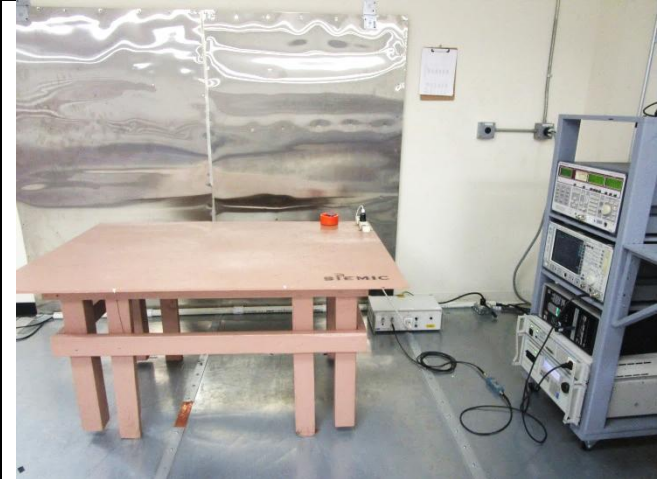
AC Line Conducted Emissions – Front View
