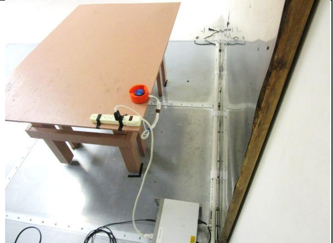
AC Line Conducted Emissions – Rear View
