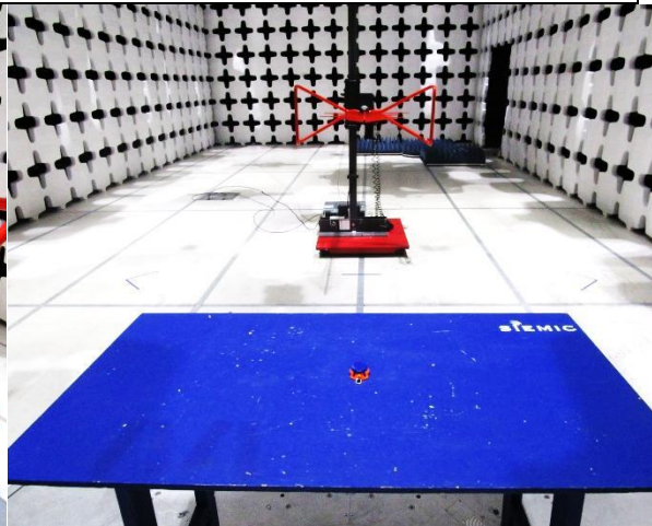
Radiated Emissions (<1GHz) – Rear View
