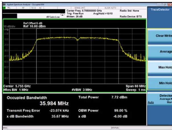
(802.11 n40) 99% Bandwidth plot on channel 159
