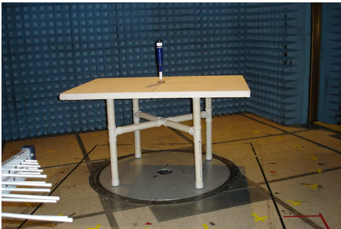
Figure 6. Photo of radiated emissions set-up used during fundamental evaluation.
