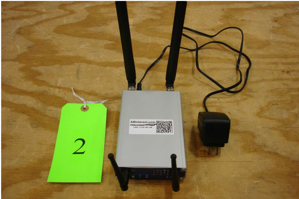
Figure 2. Auxiliary Communications Hub (see photo below for more details located on back of product)
