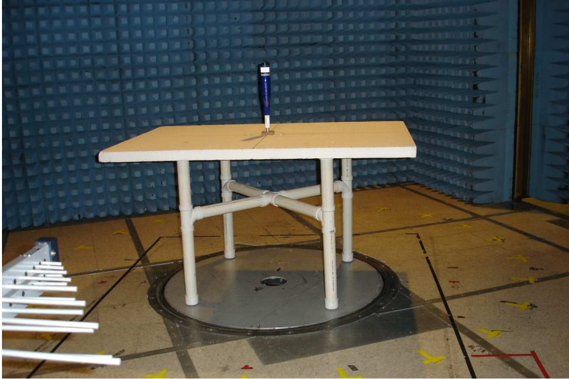
Photo of radiated emissions set-up used during fundamental evaluation.
