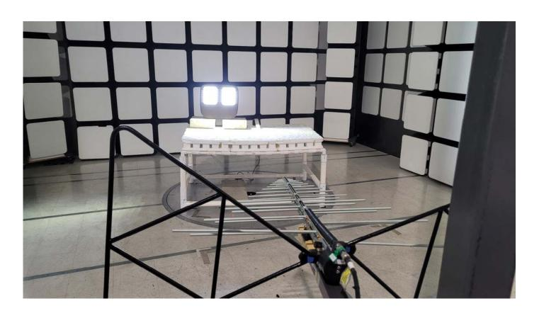
MESH SYSTEMS LLC LIGHTING CONTROL NODE MODEL: LCN300 FCC SUBPART B AND C – RADIATED EMISSIONS – BELOW 1 GHz
