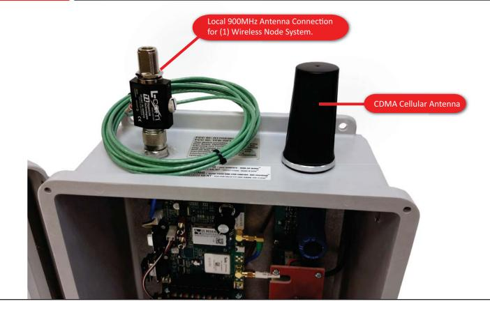
If there is more than one (1) Wireless Node in the system, you will need to install the high gain 900MHz BFA antenna and mounting bracket. The "L" bracket is designed to clear gutters. Mounting hardware and conduit is not supplied by the manufacturer.
