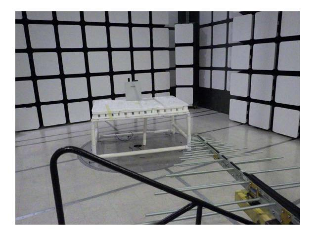
MESH SYSTEMS LLC LIGHTING CONTROL GATEWAY MODEL: LCG300 FCC SUBPART B AND C – RADIATED EMISSIONS BELOW 1 GHz – INTERNAL ANTENNA
