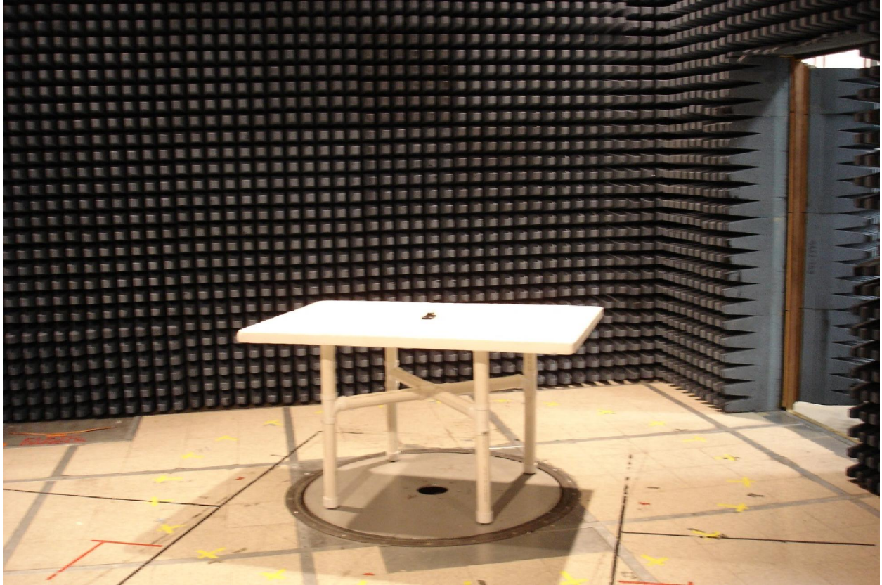
Figure 3. Radiated Emissions EUT Set-up for Frequencies < 1GHz
