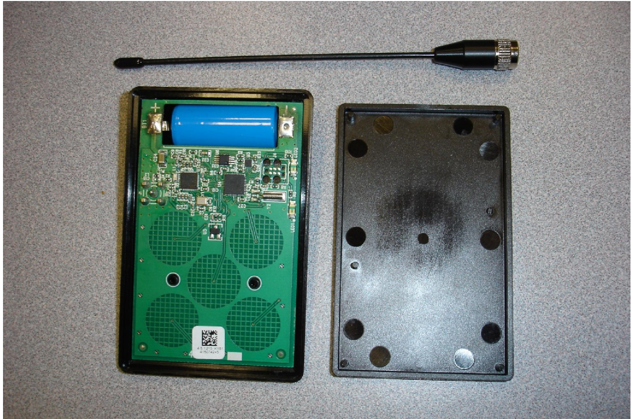
Enclosure shown opened with PCB Assembly flipped so back is up. Back cover to the side.
