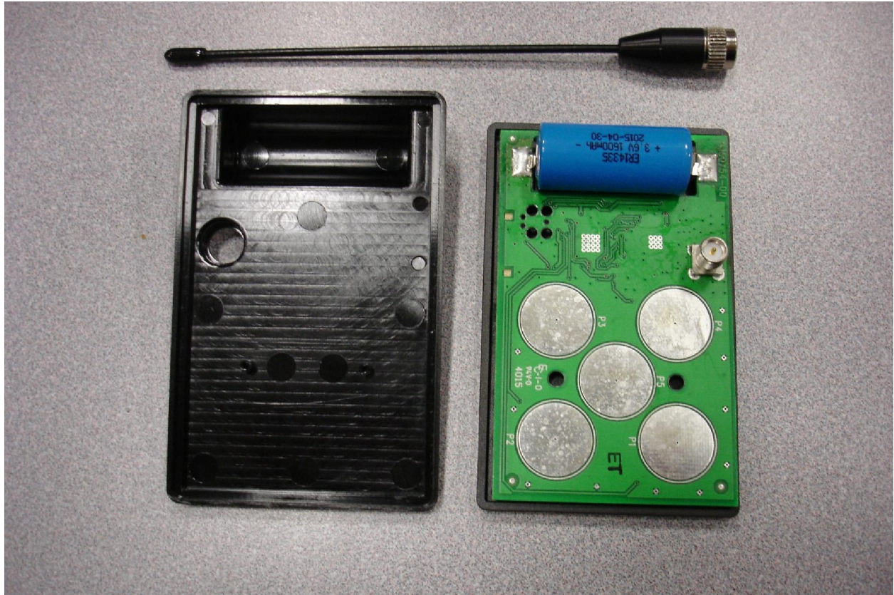
Enclosure shown opened with top of PCB Assembly shown in normal orientation.
