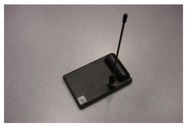
Top-side view of Sensor enclosure. Note: sticker would have coded graphic on it.
