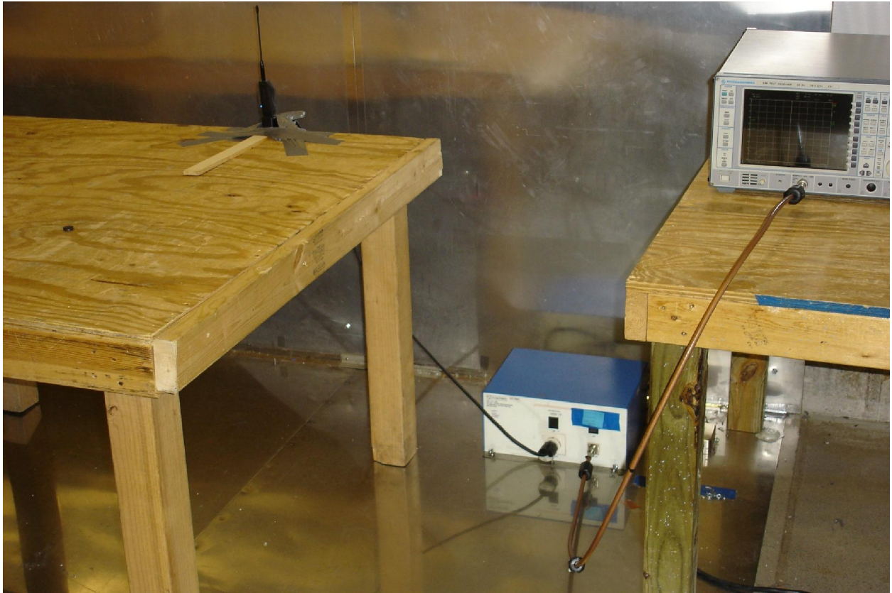
Figure 3. Powerline conducted emissions set-up (LISN)
