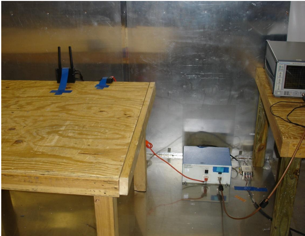
Figure 3. Photo of the Power Line Conducted Emissions Set-up.
