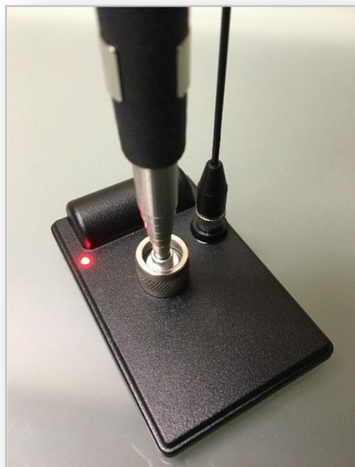
Figure 11: Sensor Light Sequence #1: RED
