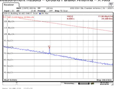
A.1. Spurious Radiated Emissions (9 kHz to 150 kHz), Fundamental = 908.4 MHz
