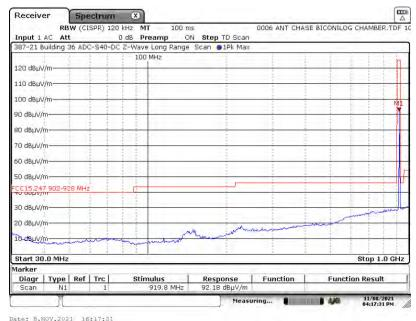
A3.2.2. Measurement Results: Vertical Antenna
