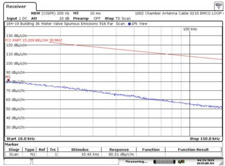
B.1.2. Measurement Results – Perpendicular Antenna
