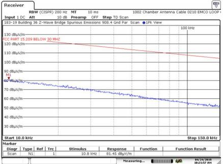
A.2. Spurious Radiated Emissions (150 kHz to 30 MHz), Fundamental = 908.4 MHz
