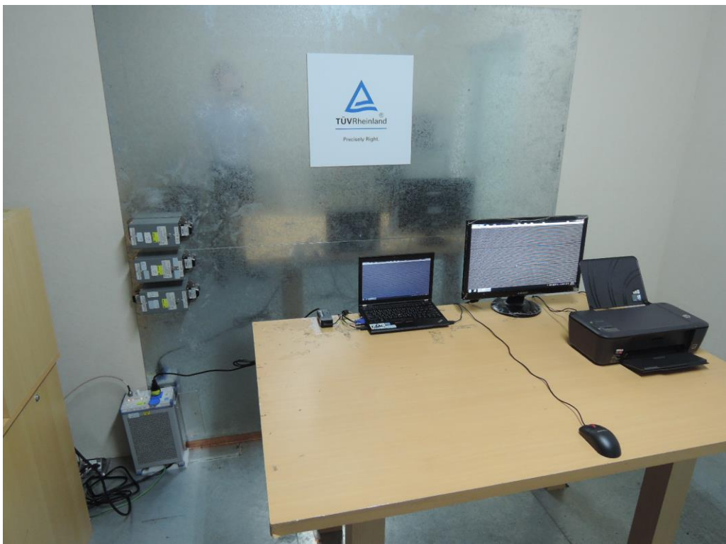
Photograph 6: Set-up for for Mains Conducted testing Front
