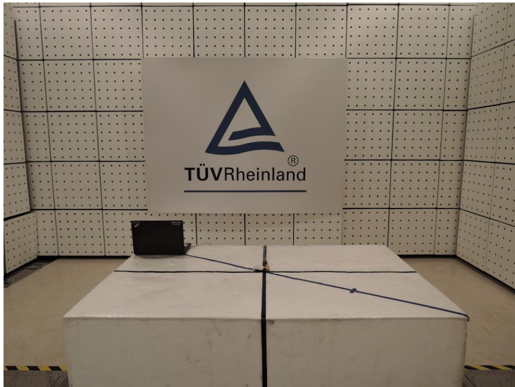
Photograph 1: Set-up for Spurious Emissions (Front View)
