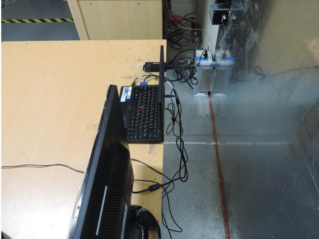
Photograph 6: Set-up for for Mains Conducted testing Front
