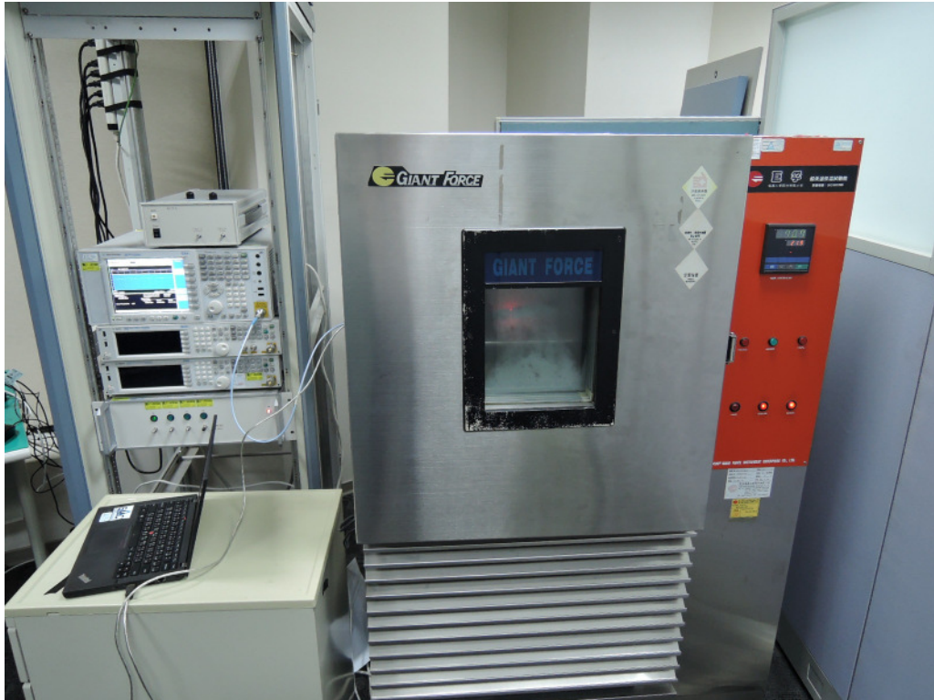
Photograph 4: Set-up for Conducted testing
