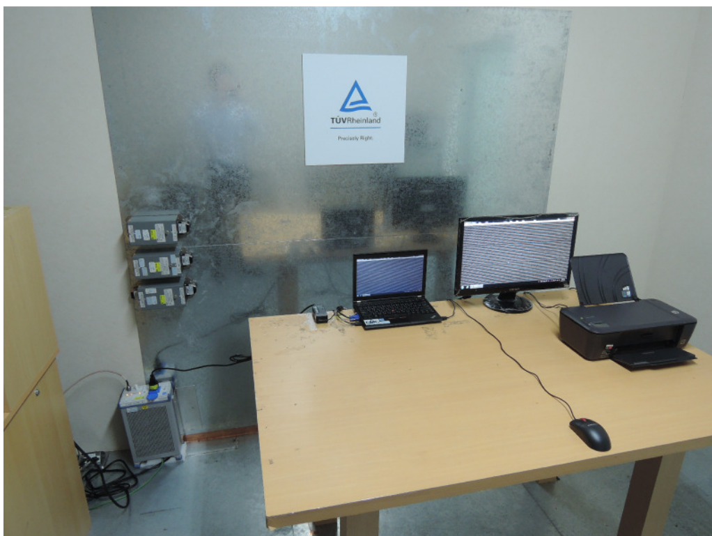
Photograph 6: Set-up for for Mains Conducted testing Front
