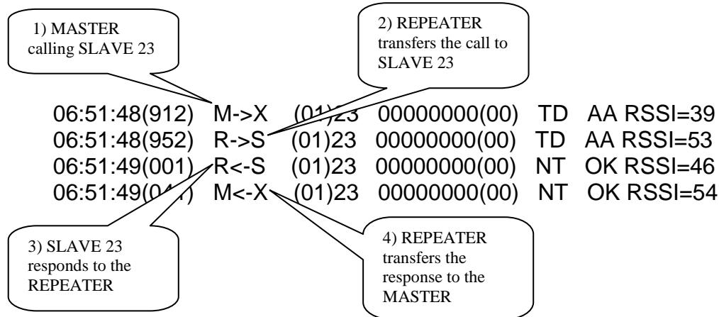
6. The recorded results are stored in text files called rfd0000.txt, rfd0001.txt, rfd0002.txt etc... Each time we exit and restart the RF EAR software a new file with a higher index is generated, thus eliminating the erasure of the previously recorded information. The following rows are taken from a file of recorded information. Notice that the first row shows the earliest record and there is exactly 100 milisec between the calls of the Master to the next RTU.
