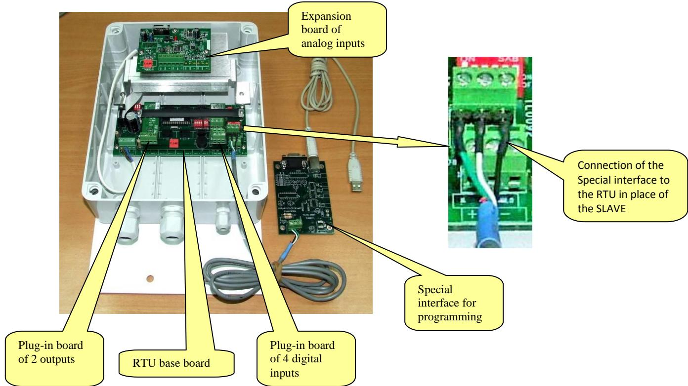
In case of sensor of 4-20 mA, a  $221\Omega$  resistor will be used as shown in the picture. Usually the board will be supplied with the resistors included. In case of 0-5v the resistors should be removed.
