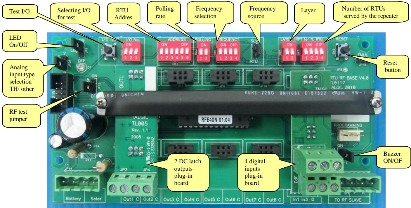
The ECONOMICAL RF RTU includes all the functions of the MODULAR RF RTU except for analog inputs and the ability of expanding the outputs.
