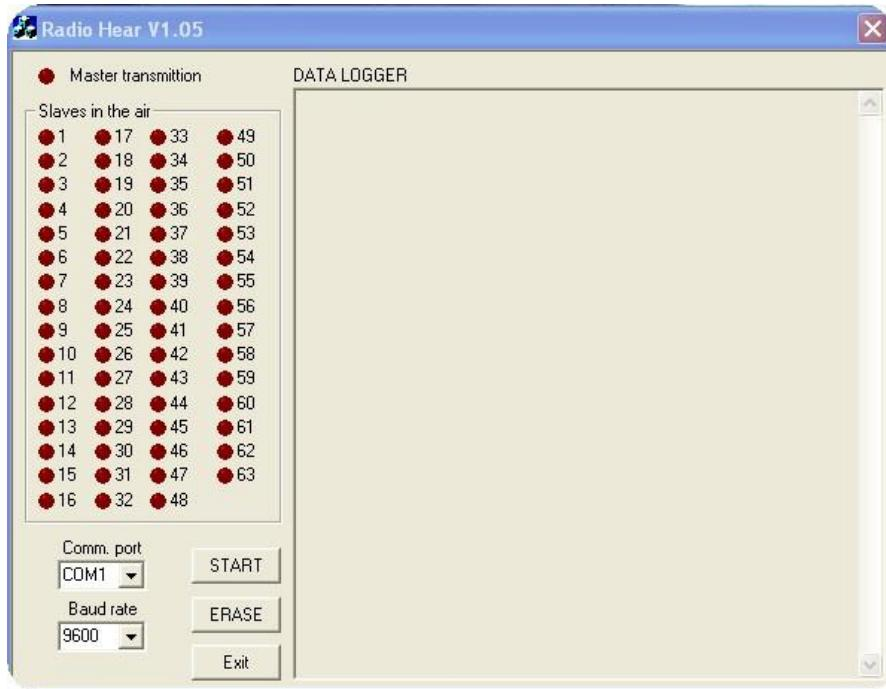
4. Connect the communication cable of the RF EAR to a serial port of the laptop, and set the “Comm. Port” of the software accordingly. For those laptops having no serial port, a USB port with a converter from USB to RS232 can be used. For GIII the Baud rate setting should be 9600 while for GIV and GIV.V it should be set to 19200.
