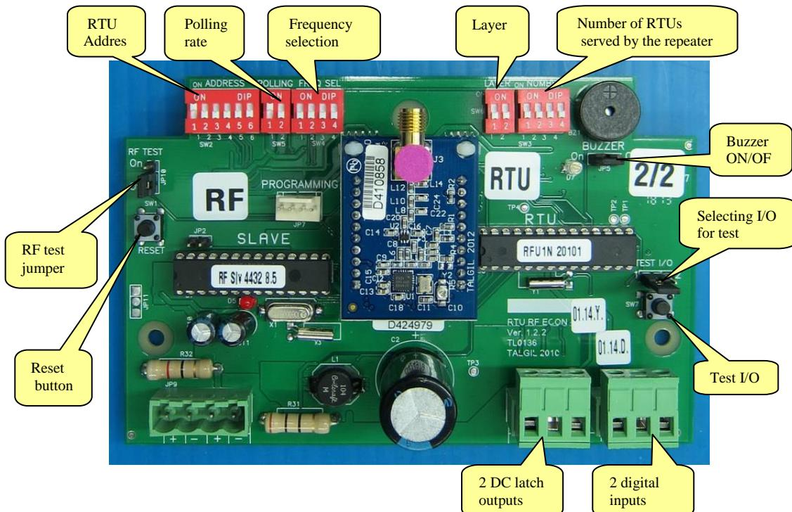
Before being able to use the RTU there are some necessary settings to be done:
