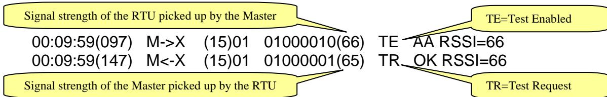
The MASTER will remain in TEST mode until receiving an END OF TEST signal from the RTU (as a result of removing jumper 15) or until the RF TEST is disabled by the user at the host controller.
