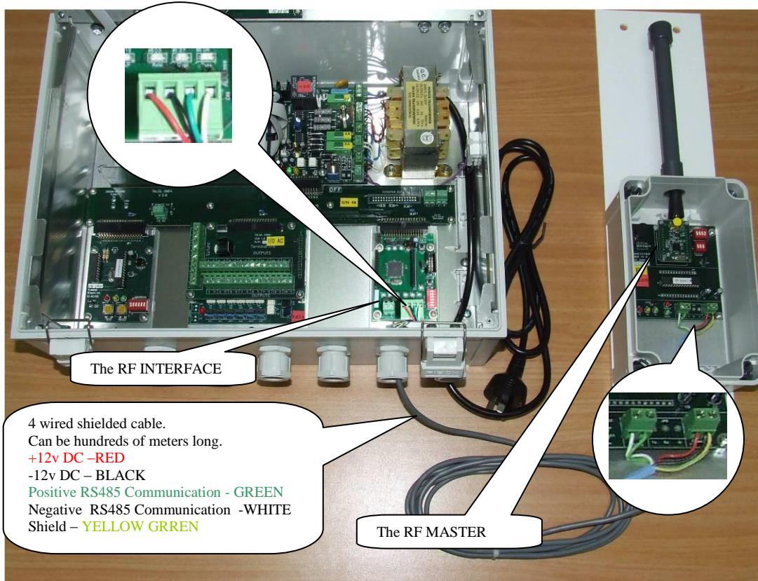
Wiring between DREAM – RF INTERFACE (internal) and RF MASTER
