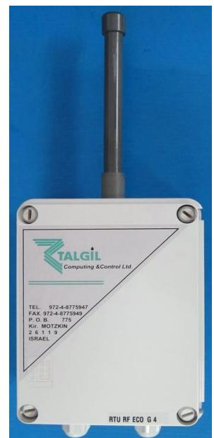
For practical reasons the Economical RF RTU cannot be installed in a too high position, because then the wiring of the outputs and inputs will be too difficult. On the other hand if we install it in a low position we shall sacrifice the height of the antenna. In order to solve this problem we use an antenna extension kit:
