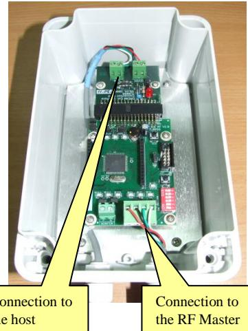
Out in the field, each RTU BASE (EXECUTER) and its RF SLAVE counterpart will also be installed on a pole with the SLAVE unit on top of the pole and the RTU BASE about 1 meter above ground. Here again the upper part of the pole, where the RF slave is located, should be of nonmetallic material and here too the connection between the SLAVE and the RTU BASE uses a shielded 4 wired cable.
