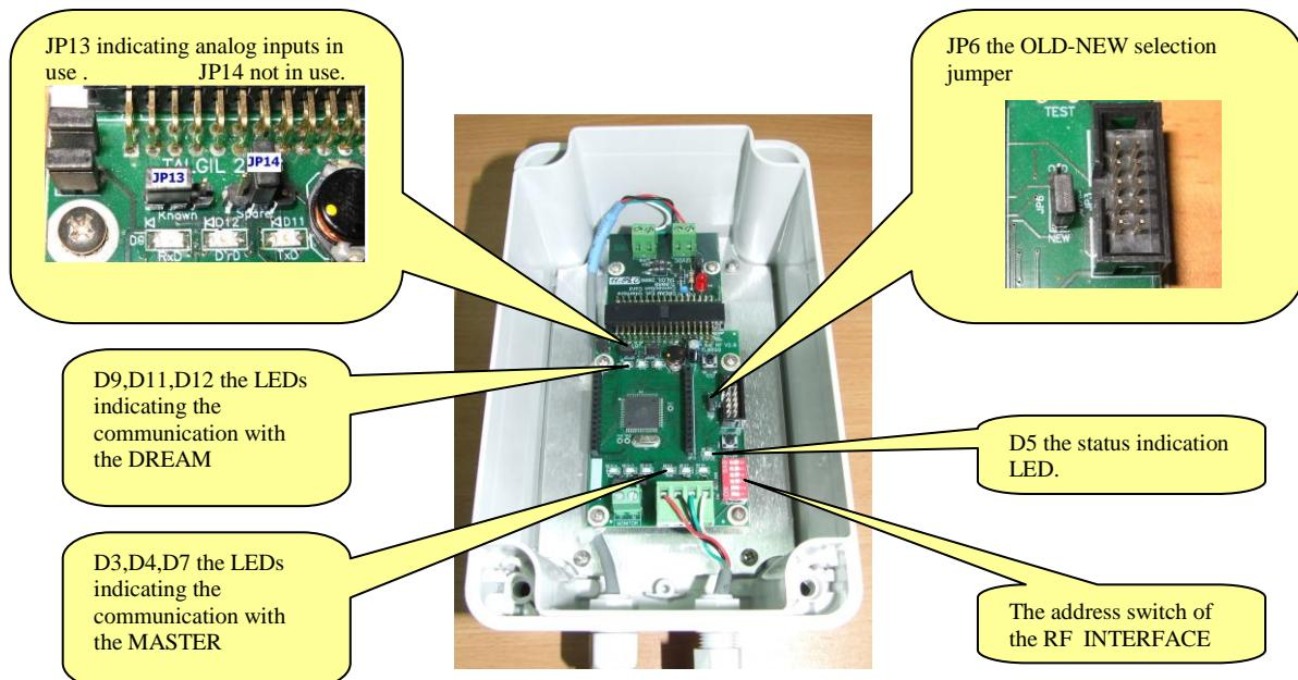
Setting the channel address is done by use of the Address Dip Switches. The address must be set according to the address defined at the DREAM (or other host) controller. Make sure that there is no other interface with the same address. Notice that the addressing uses binary coding. See “Appendix A” about the binary to decimal conversion.
