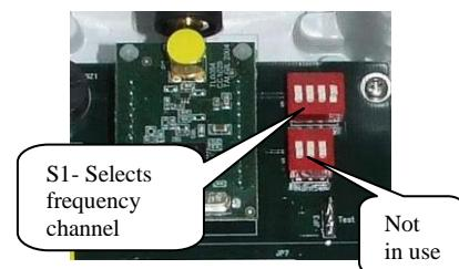
2. Turn on the power switch of the RF EAR. The unit will start sounding sequences of short beeps repeated in an interval of the scanning rate. Each short beep indicates a communication picked up by the unit.
