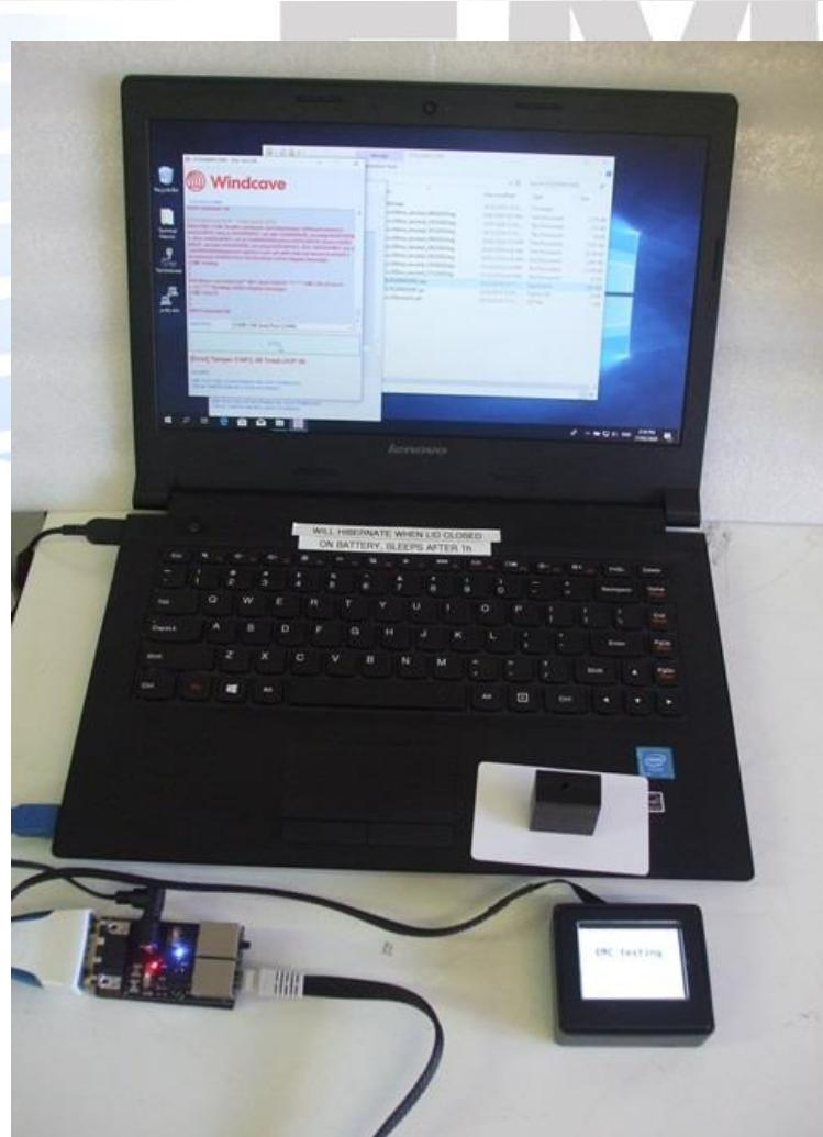
Conducted emissions test set up
