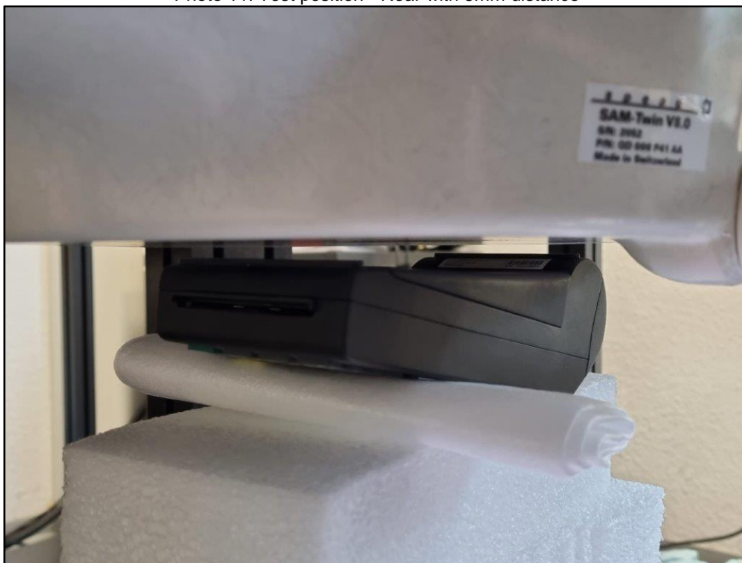
Photo 12: Test position - Bottom with 0mm distance
