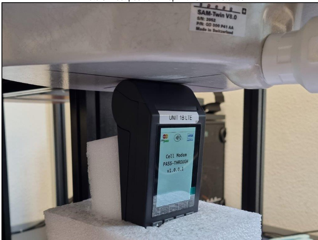
Photo 8: Test position - Top with 0mm distance
