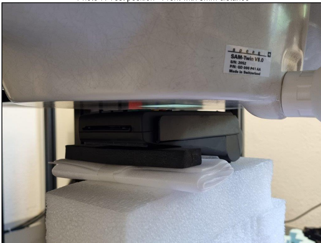
Photo 8: Test position - Top with 0mm distance
