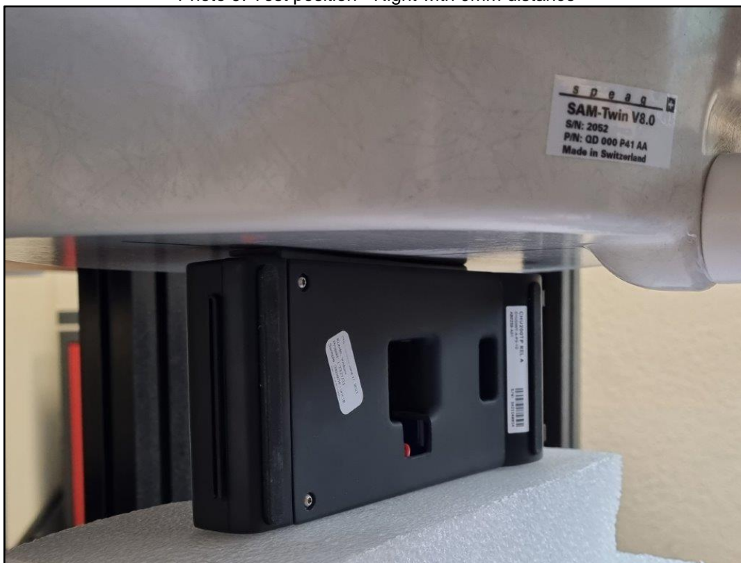
Photo 10: Test position - Rear with 0mm distance
