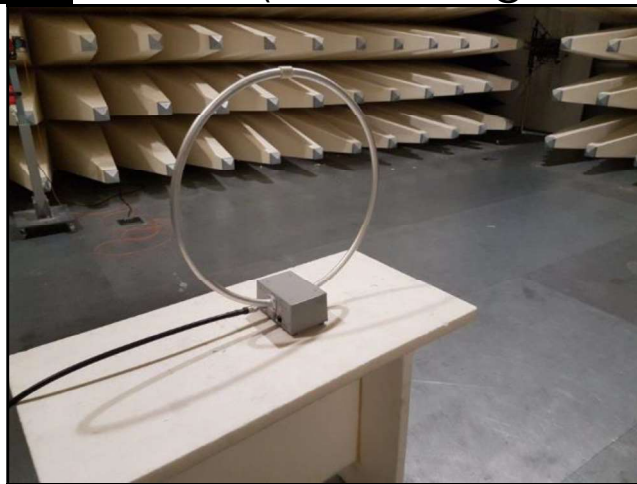
Loop-Antenna: EMCO 6502A (Correction factor @ 13.56MHz +9.5 dB)
