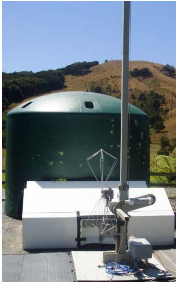
Test Shed showing the use of a Biconical Antenna
