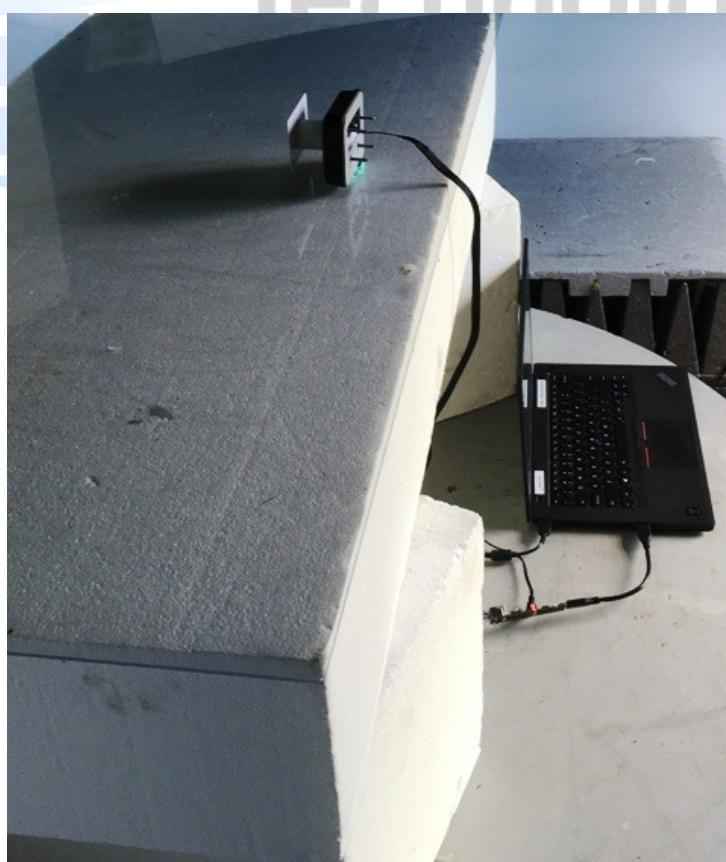
Conducted emissions test set up
